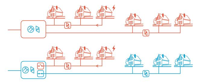
The failing segments can be segregated with ingress switches.
