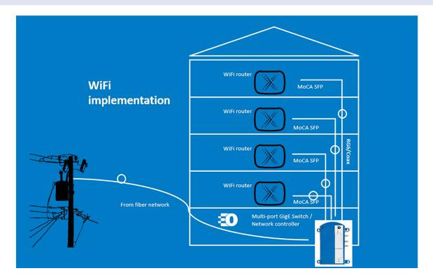
The Intercept™ **EO** is full featured and targeted to the Multi Dwelling Unit market segment for high speed symmetrical data services in a compact and versatile design which supports up to 31 subscribers per RF port.
