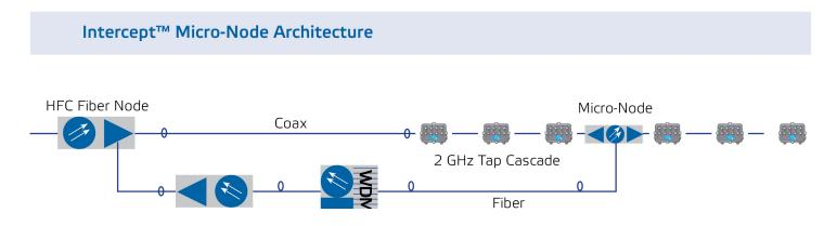
Traditional HFC network architectures must be re-considered in order to meet these new demands of high frequency operation to 1794 MHz. In many cases where cable spans are stretched, current HFC architectures will not meet CPE input levels as designed, or required CNR and linearity for an economically and technically viable transition to full band 1794 MHz operation.
